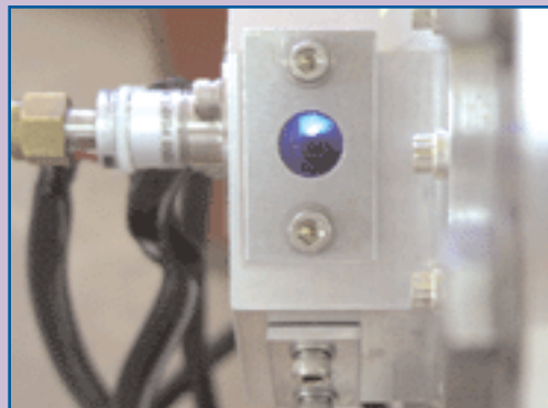
Plasma portal. Through a small window in the deposition tool, operators can view the plasma plume created by the laser ablation pulse focused down on a target metal surface.
